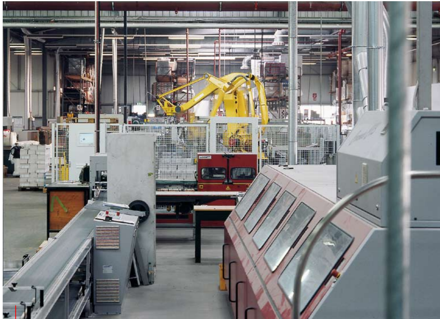
A second RS 400 palletizing robot has been added to the existing robot cell. Now the complete palletizing process behind the two perfect binder lines is fully automated with a double-robot solution.
