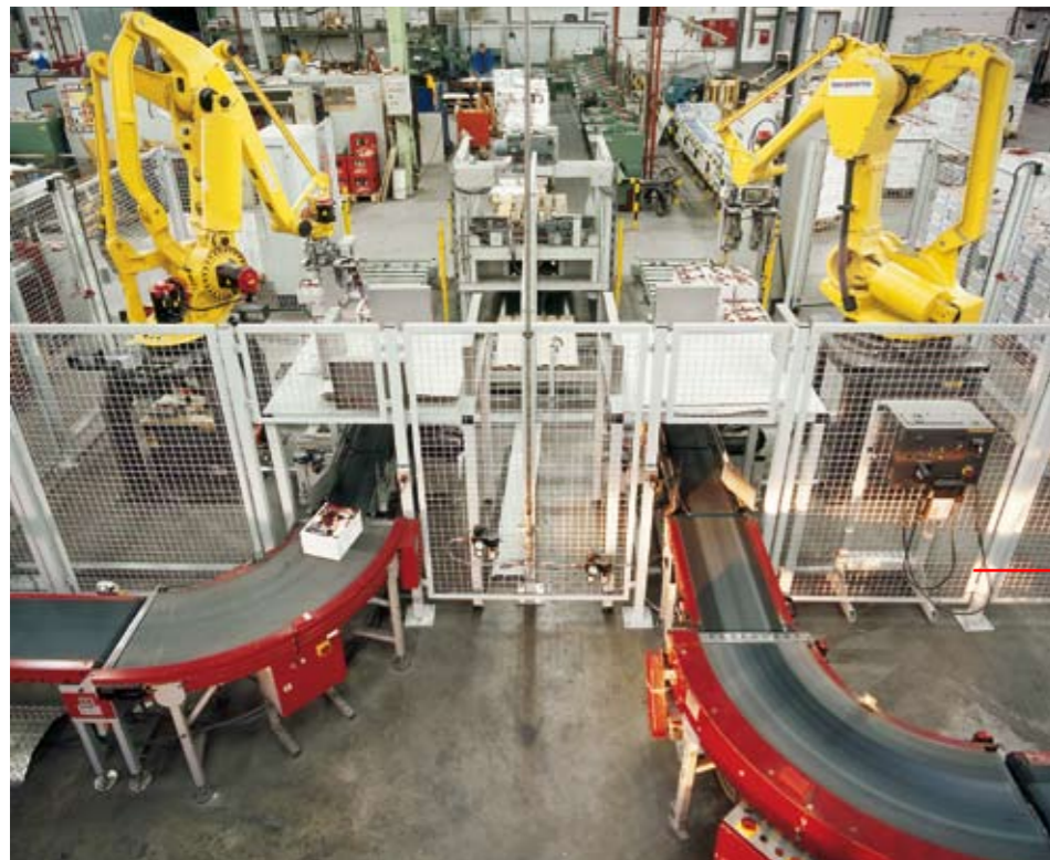
The stacks are transported by two stack conveyors from the perfect binder lines to the pick-up stations of the palletizing cell. Two RS 400 robot arms equipped with double grippers pick up the loose stacks and place them smoothly on the automatically delivered pallets. The palletizing cell processes up to 2000 stacks/h.
