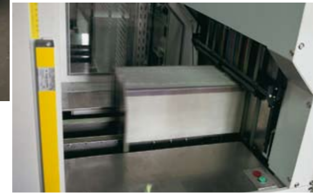
▲ The RS 600 builds stacks of 800-1200 mm length at a speed of up to 80,000 cph. Innovative details like CST („Continuous Stacking Technology“), a floating stacking head and swords with air stream ensure an excellent log quality. The great ergonomics of the RS 600 improve safety and operation (operation can be done from one side), allows easy visual control and free access to the stacking area.
