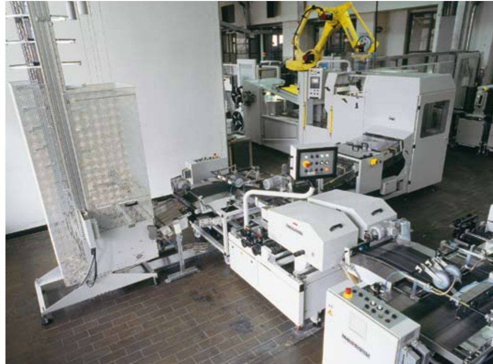
Within the stack and log building area the shingled stream goes via a second divert gate either directly to the RS 600 log stacker or can alternatively be directed to an RS 820 trimming
