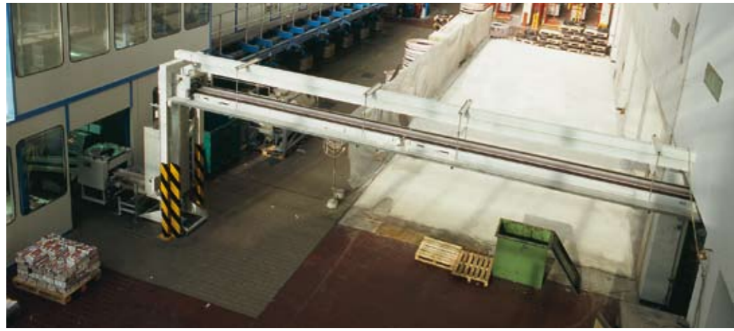
◀ The products are transported from the pressroom via an overhead conveyor to the post press area. According to demand an integrated divert gate within the overhead conveyor makes it possible to transport the products either to a print roll system or to the stacking and log building area.
