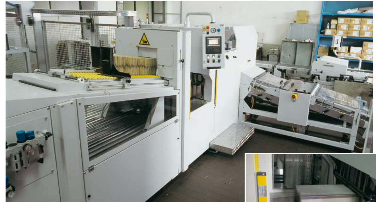
◀ The products are transported from the pressroom via an overhead conveyor to the post press area. According to demand an integrated divert gate within the overhead conveyor makes it possible to transport the products either to a print roll system or to the stacking and log building area.
