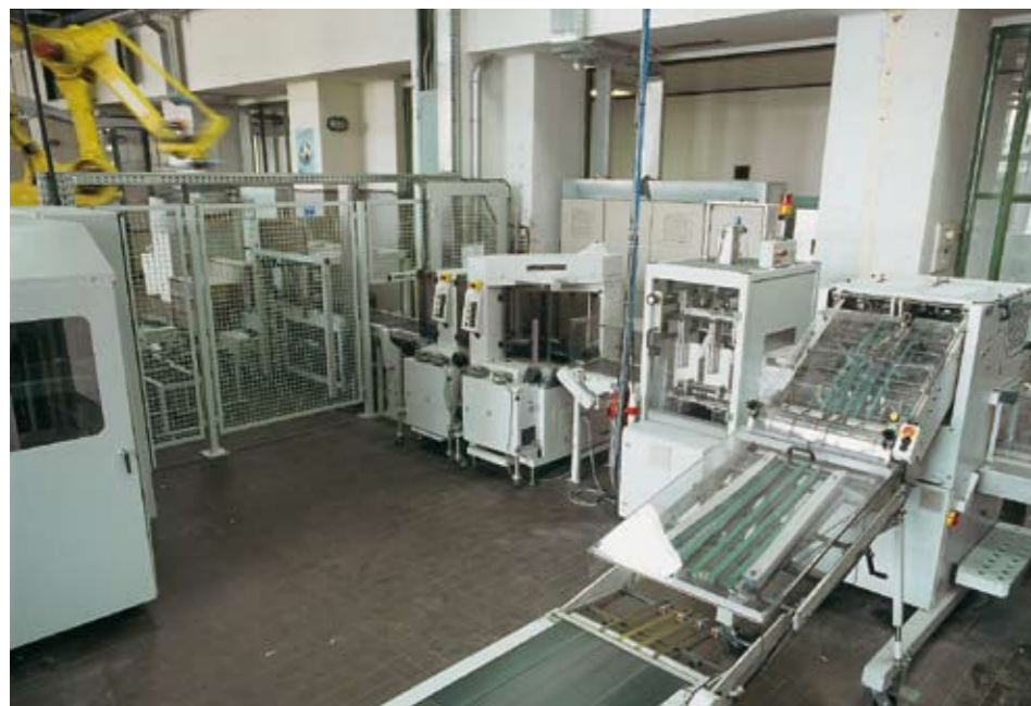
◀ After the three-side trimming the products are directed to an RS 32 compensating stacker. The perfect stacks are then compressed and stabilized by an electrostatic charge by the direct-coupled blocking unit RS 100. Before palletizing the stacks are single-, double- or cross-strapped.
