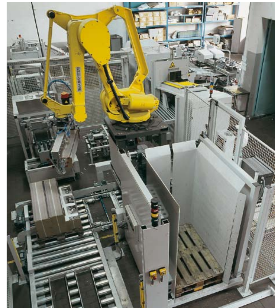
▲ The RS 600 builds stacks of 800-1200 mm length at a speed of up to 80,000 cph. Innovative details like CST („Continuous Stacking Technology“), a floating stacking head and swords with air stream ensure an excellent log quality. The great ergonomics of the RS 600 improve safety and operation (operation can be done from one side), allows easy visual control and free access to the stacking area.
