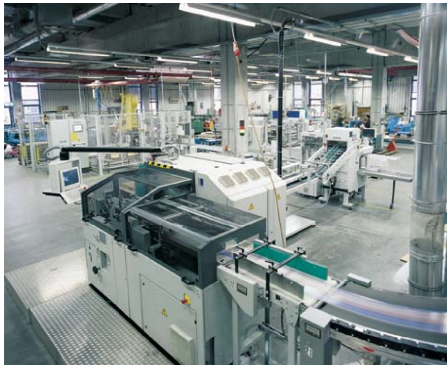
▲ The RS 33S bookbindery stacker especially designed for thick products receives the perfect bound and trimmed products (up to 80 mm product height). Equipped with the „table-up option“ which reduces the drop height between the upper bin and lower turntable basket the RS 33S produces perfectly aligned stacks.
