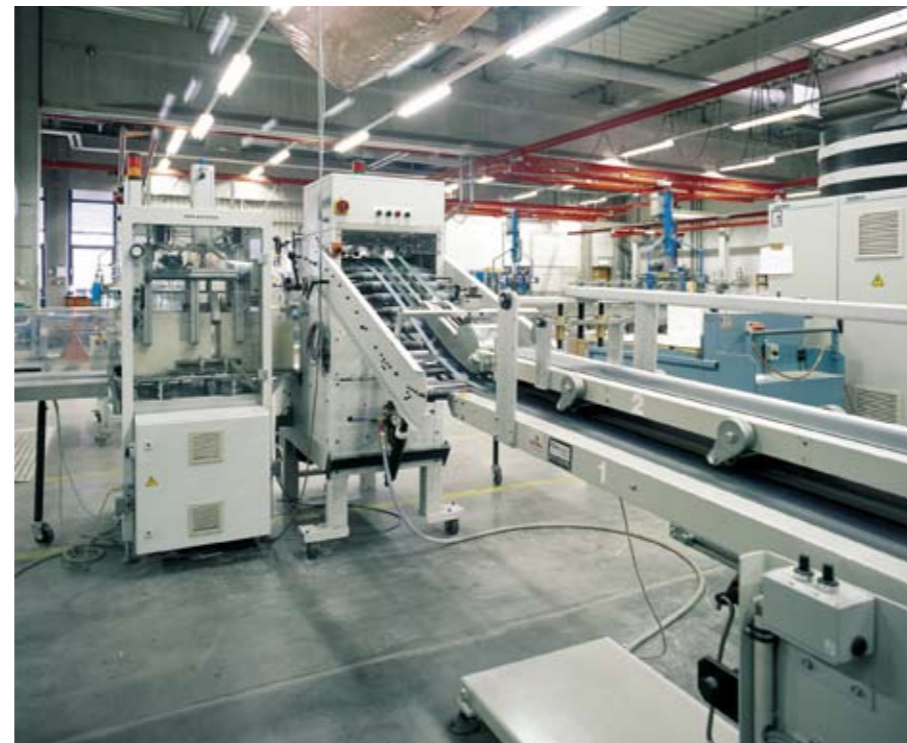
▲ The high speed pusher system of the RS 33S delivers the stack within the shortest cycle times to the close coupled blocking unit where the stack is stabilized through mechanical compression and an electrical charge for safe transport and palletizing.
