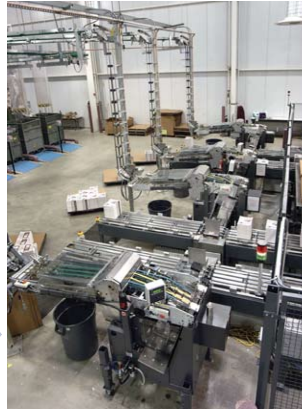
▲ The four streams of the PFF 2 folder are redirected to spine leading orientation and transported to the RS 50S stackers via four overhead conveyor lines. This clears the floor space and guarantees fast and direct access to all machines.
