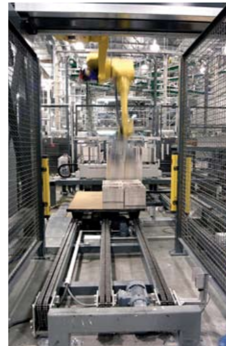
▲ The RS 500 robot palletizes from four lines onto four pallets. Pallet handling and slip-sheet feeding are fully automatic. If necessary one robot can also serve all four lines giving the system unique productivi-
