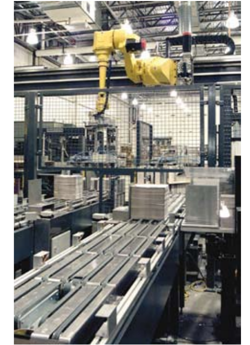
▲ The compressed, brick like stacks from the RS 50S are transported to the pick-up stations. The reverse mode of the stack conveyors allows manual pick-up of sample stacks and can be used as additional stack buffer.
