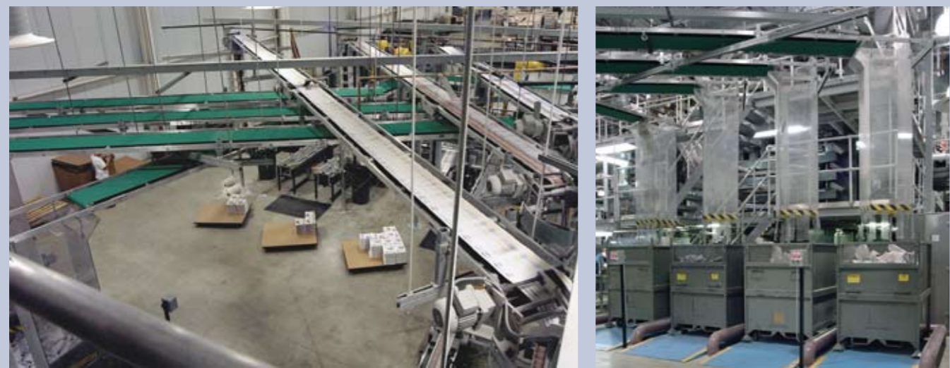
The divert gates for the waste copy ejection are part of the overhead section. The waste copies of each line are collected and delivered in a separate waste bin. This allows detailed analysis of printed and waste copies.
