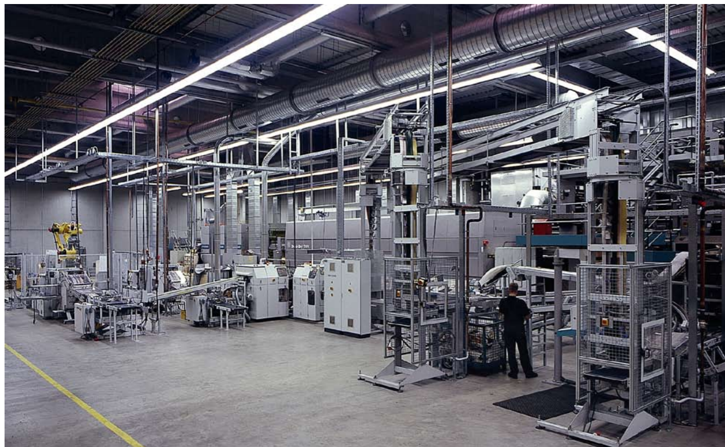
Automated Post Press solution for a one man operation: conveying system with overhead- and floor conveyors, RS 840 double stream trimming line, two RS 31SL stackers with close coupled blocking unit and strapping unit and RS 400 high speed palletizing robot with double and multi gripper.
