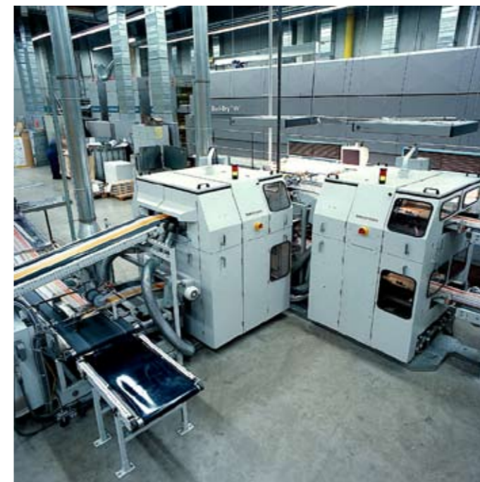
The innovative RIMA-SYSTEM double stream trimmers represent a space saving and easy accessible solution for three side trimming of two shingled streams. The two trimming modules operate separately and can be run together or individually. All format adjustments are electrically controlled by the commander of the RS 840.
