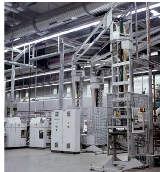
The overhead conveyors transport the shingled streams to the RS 840 double stream trimmers. The RS 300 overhead conveyors guarantee the operator fast and easy access to the deliveries and to the complete Post Press System.
