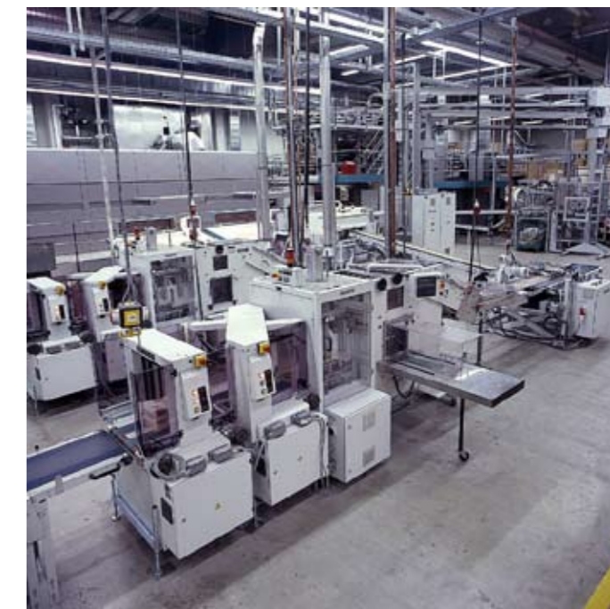
After the three side trimming, each shingled stream is delivered to a RS 31SL high speed stacker. The closed coupled blocking unit stabilizes the stacks by applying electrostatic charges. The stacks can optionally be single or cross strapped. Loose stacks run through the in-line strapping line.
