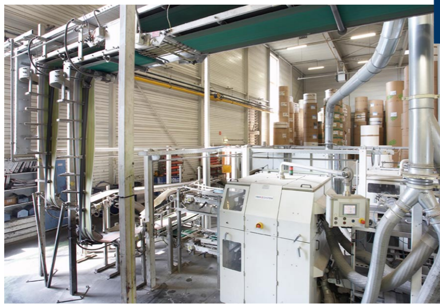
The production of the folder deliveries is transported via overhead conveyors to the RS 840 double stream trimming line for three side trimming. Alternatively, products can bypass the trimming line without trimming. The RS 840 is equipped with an electrical format adjustment and guarantees a precise cut thanks to proven features like Hexbrator Technology and integrated knife cooling. Before trimming or bypassing the trimming line, start-up, blanket washing and splicer waste is ejected.
