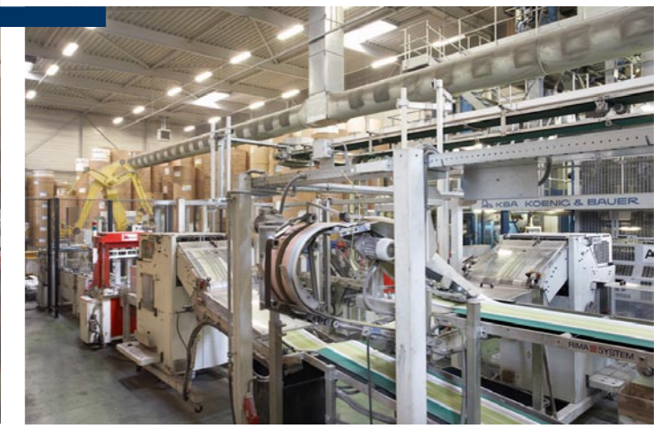
Trimmed or untrimmed productions are directed to the RS 32 high-speed stackers. Spiral conveyors guarantee the space-saving and secure transport of products without any shift of copies. Each stacker turns up to 120.000 cph into neat stacks which are ejected by an intelligent servo-pusher system onto the synchronized delivery belts
