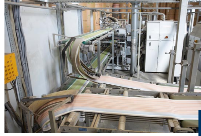
Trimmed or untrimmed productions are directed to the RS 32 high-speed stackers. Spiral conveyors guarantee the space-saving and secure transport of products without any shift of copies. Each stacker turns up to 120.000 cph into neat stacks which are ejected by an intelligent servo-pusher system onto the synchronized delivery belts
