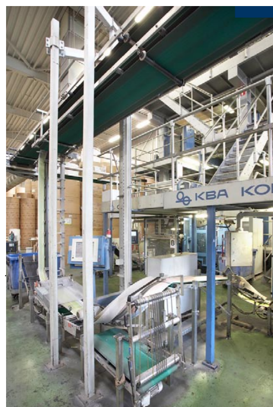
The production of the folder deliveries is transported via overhead conveyors to the RS 840 double stream trimming line for three side trimming. Alternatively, products can bypass the trimming line without trimming. The RS 840 is equipped with an electrical format adjustment and guarantees a precise cut thanks to proven features like Hexbrator Technology and integrated knife cooling. Before trimming or bypassing the trimming line, start-up, blanket washing and splicer waste is ejected.
