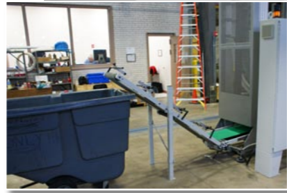
The shingled streams of the two A3 (tabloid) and A4 (quarterfold) folder deliveries are directed via floor conveyors to a central waste ejection system where start-up, blanket wash and splice waste is ejected. Good copies run into the heavy-duty upward conveying tower for newspapers.
