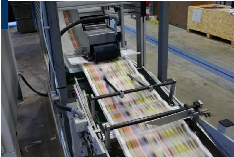
The specially developed c-shaped upward and downward conveying towers enable the secure and space-saving transport of newspaper products. Between extra robust belts the shingled stream is transported 90° upward without any twist and is conveyed as an inverted shingle to the downstream equipment.
