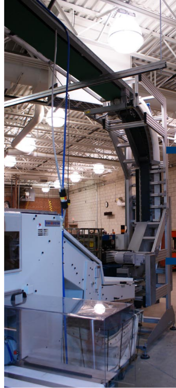
The inverted shingled stream is transported via overhead conveyors to the c-shaped conveying tower which directs the products 90° downward and directly into the RS 36 indexing stacker for newspapers. The RS 36 turns the shingled stream into neat stacks. Even products with high pagination are perfectly compressed and ejected via a servo-pusher system with fully synchronized delivery belts to an air-operated delivery table.
