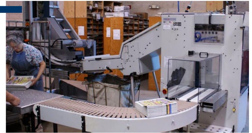
The inverted shingled stream is transported via overhead conveyors to the c-shaped conveying tower which directs the products 90° downward and directly into the RS 36 indexing stacker for newspapers. The RS 36 turns the shingled stream into neat stacks. Even products with high pagination are perfectly compressed and ejected via a servo-pusher system with fully synchronized delivery belts to an air-operated delivery table.
