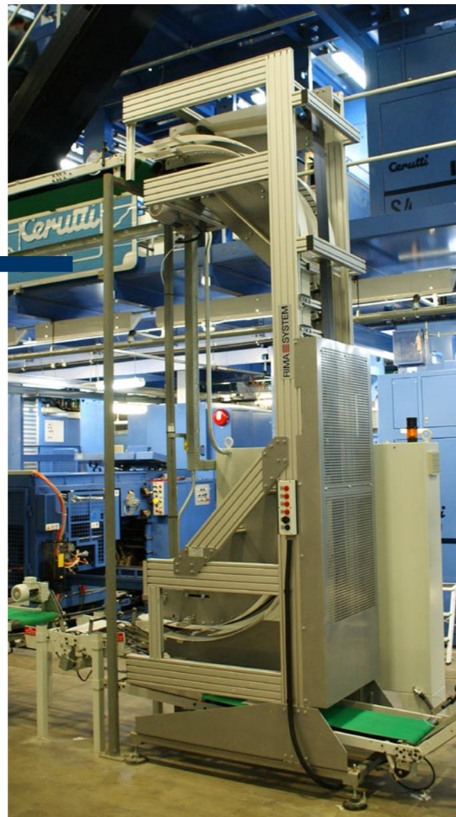
The specially developed c-shaped upward and downward conveying towers enable the secure and space-saving transport of newspaper products. Between extra robust belts the shingled stream is transported 90° upward without any twist and is conveyed as an inverted shingle to the downstream equipment.
