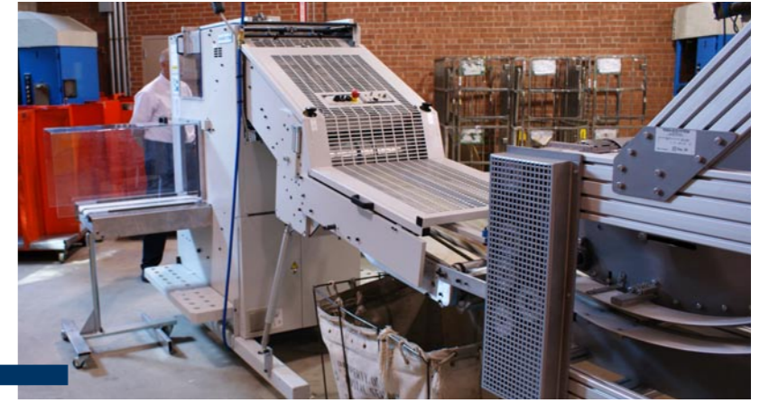
The inverted shingled stream is transported via overhead conveyors to the c-shaped conveying tower which directs the products 90° downward and directly into the RS 36 indexing stacker for newspapers. The RS 36 turns the shingled stream into neat stacks. Even products with high pagination are perfectly compressed and ejected via a servo-pusher system with fully synchronized delivery belts to an air-operated delivery table.
