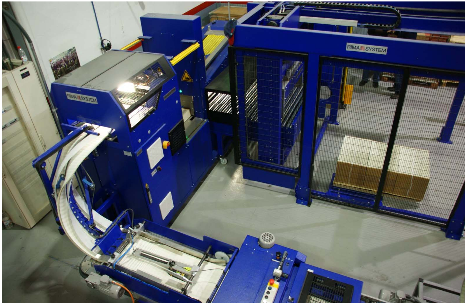
Top view of the RS 610 log stacker with RS 655 log palletizer
