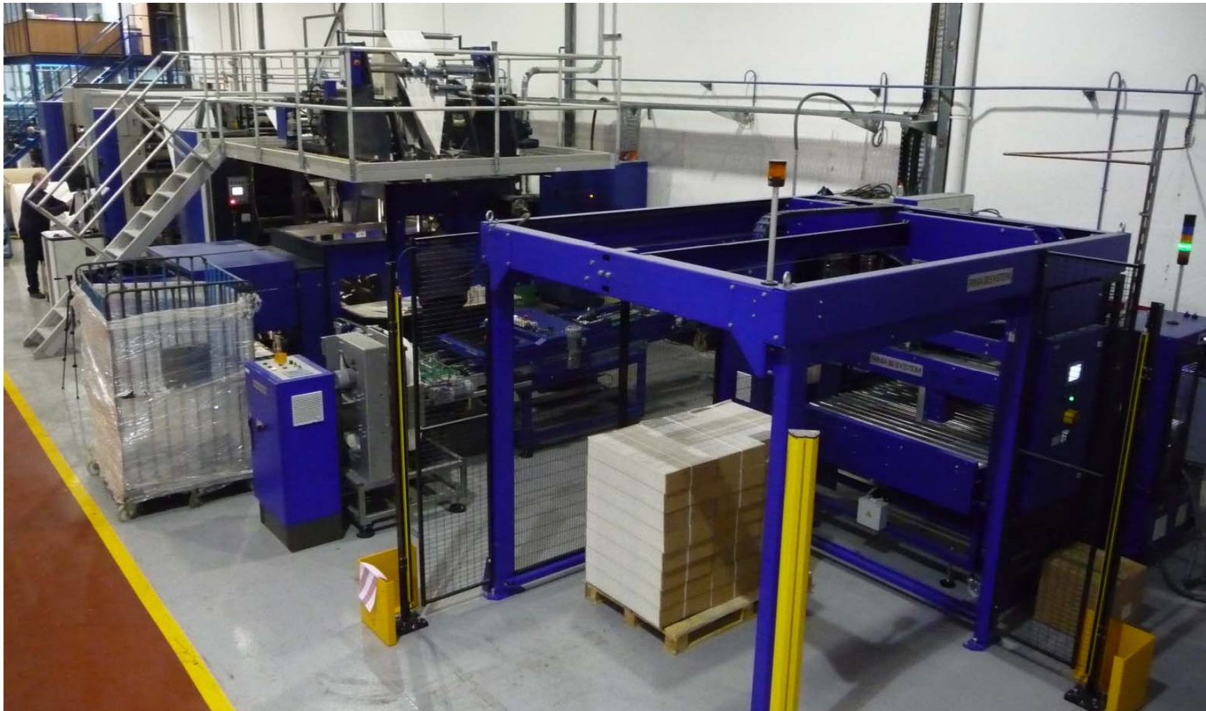
View of the Post Press solution including floor conveyors, RS 610 log stacker and RS 655 log palletizer.
