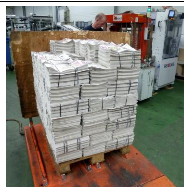
...and high speed (stitched @ 60.000cph). The RS 36S is perfect behind medium to high speed newspaper presses.
