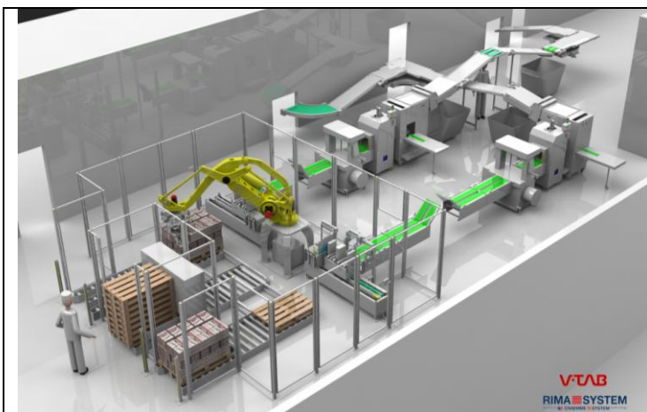
Fully automated solution in newspaper: two lines after a DGM coldset press are handled by RS 36S newspaper stackers and an RS 400 palletizing robot.
