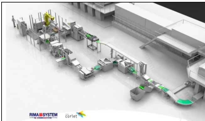
The fully automated Post Press system at Corlet Roto: products can be either trimmed and stacked or can enter the RS 610 log stacker and the RS 36S indexing stacker untrimmed.
